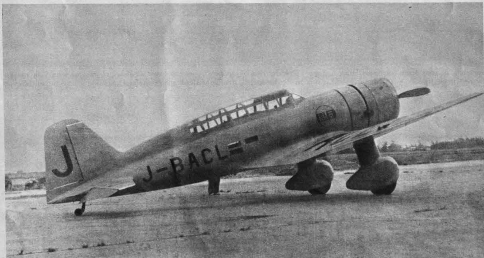
Babs, like Ann (top), is a retired reconnaissance type. It was developed from commercial plane "Kamikaze" which made a record Tokyo-London flight in 1937. Later version (above) was a two-seater with a long, faired greenhouse. Fixed landing gear is covered with large spats.
